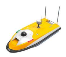
The THURN USV Profiler System provides all the tools for your USV sub bottom requirements. Supplied with a GeoAcoustics GeoPulse compact and an SBG INS/positioning sensor all of which come fully integrated. The system was designed to enable remote surveys, keeping people out of the water and minimising risk.
